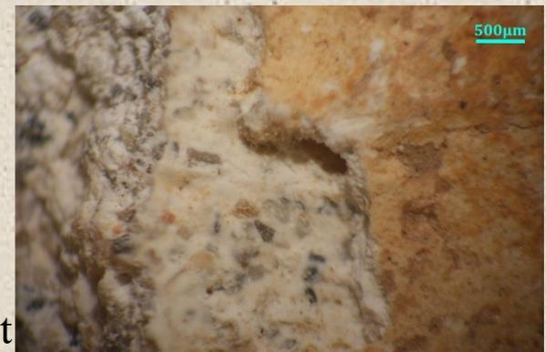
Optical microscopy of cross sections and the re-designed mortar profiles to measure the mortar aggregate grain size. A very compact microstructure was observed explaining the mortar longevity.
