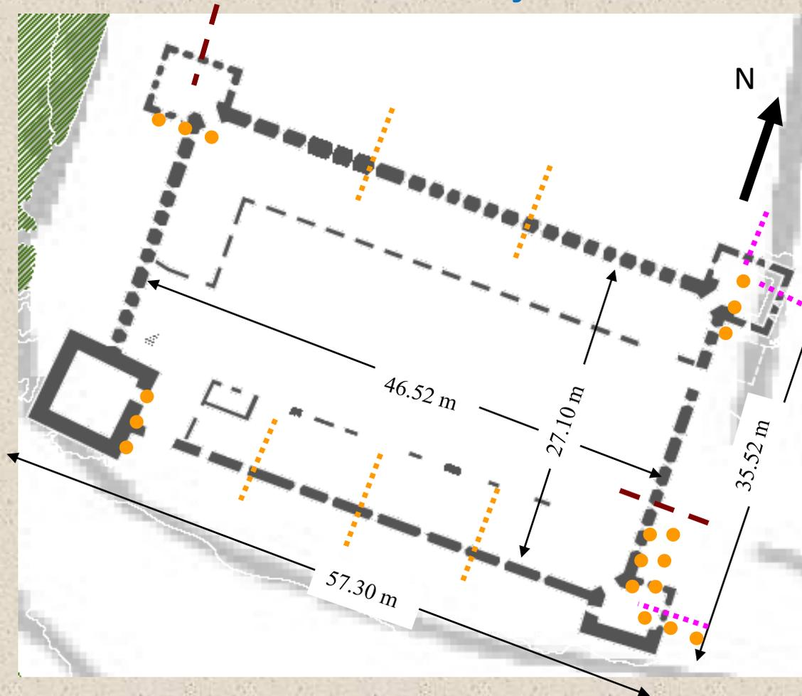
The three towers, northwest, north-east and south-east has an average height of 9 meters. The southwest tower is higher, 15 meters and has a larger base.
